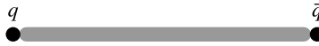
Fig. 13.10 Between a static quark–antiquark pair a flux tube develops and leads to a linearly rising potential
